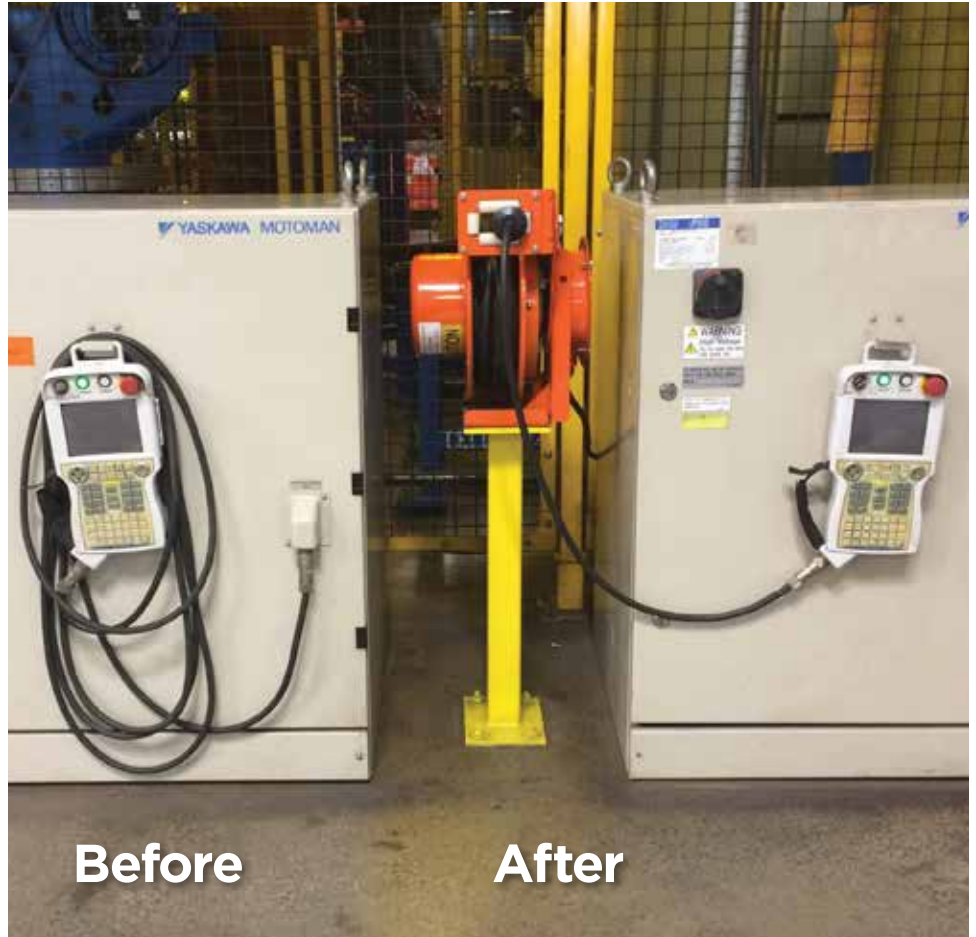
Shown is a Motoman DX100 pendant cable reel
